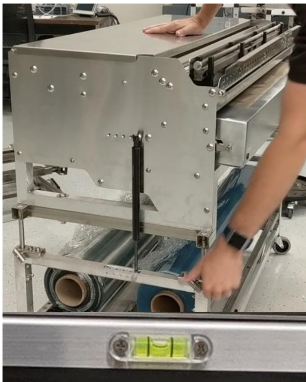
4. While maintaining desired height, lock one side of the unit to secure. Using the Height Level on the front center of the unit, adjust opposite side until the level bubble is centered in the vial then lock securely in place.
