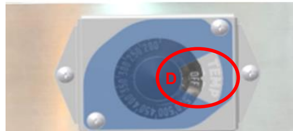
Thermostat Dial with Tamper Guard Recommended start temp: 200 degrees
