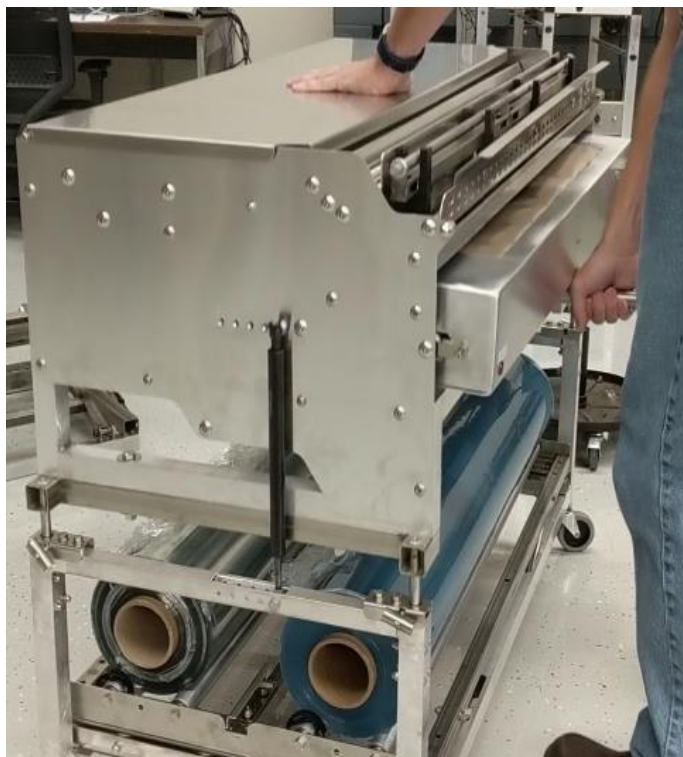
3. Using Height Adjust Handle for leverage, push down on center of Work Surface Lid to lower or lift handle to raise to desired height.
